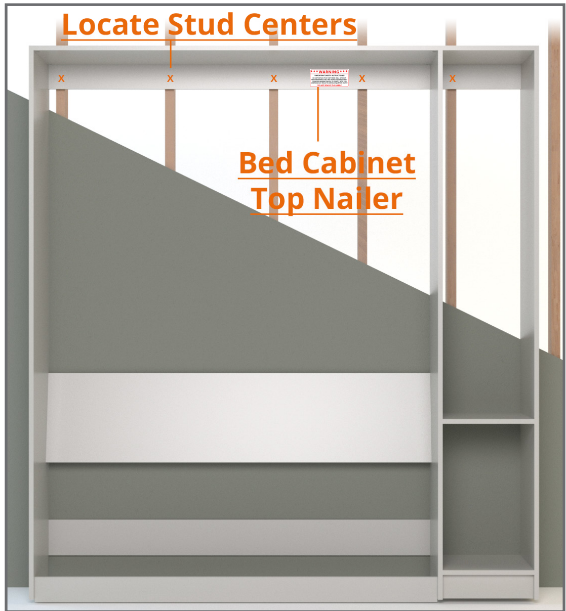
FIG. 3A - DRYWALL CUTAWAY SHOWING WALL STUDS
