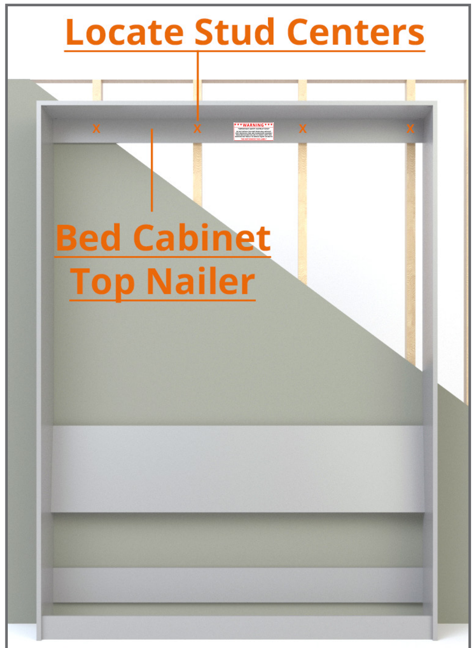
FIG. 3A - DRYWALL CUTAWAY SHOWING WALL STUDS
