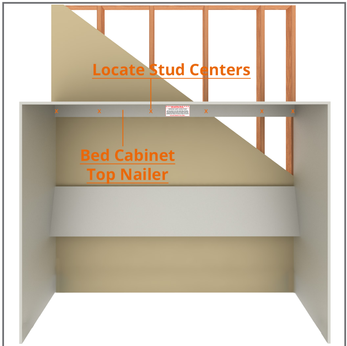
FIG. 3A - DRYWALL CUTAWAY SHOWING WALL STUDS
